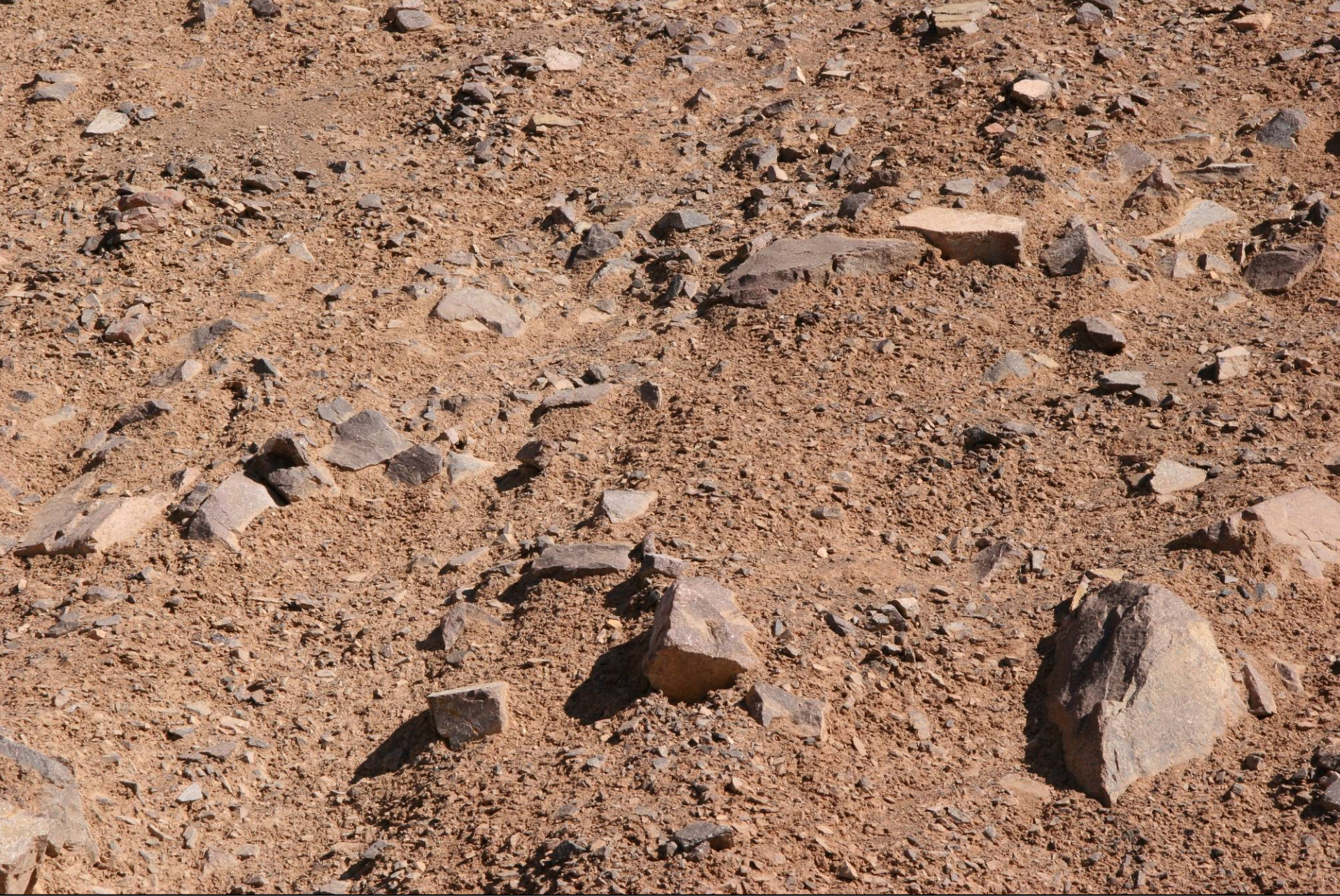
Close up of “dirty” rockfill exposed at failure site. For scale, the large rocks are 10-12” in diameter.
