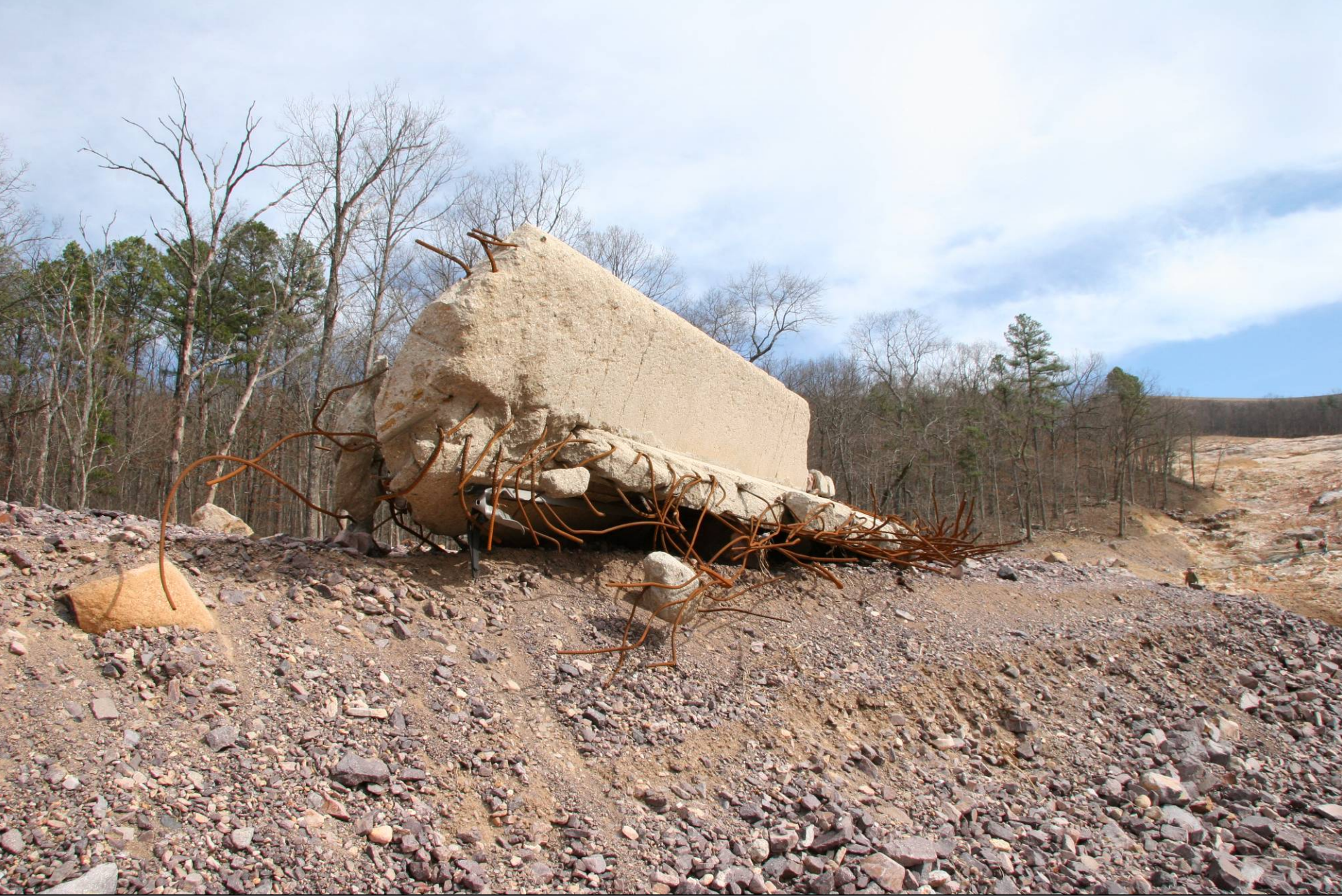
Huge pieces of rock and concrete were carried down the slope by the turbid debris flow. A large section of a concrete wall panel is shown here.
